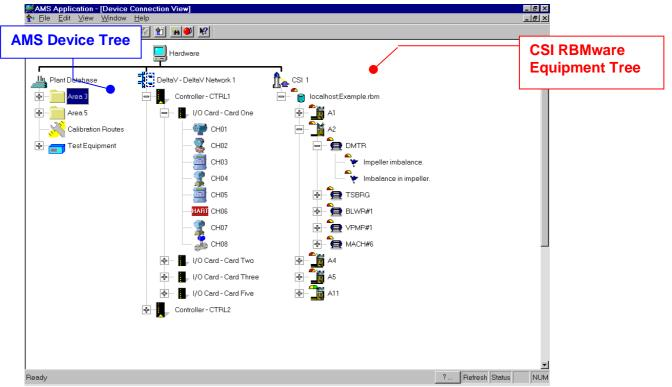
Figure 2. Process instrumentation and rotating equipment information is displayed jointly in a single user screen with the AMS/RBMware interface
