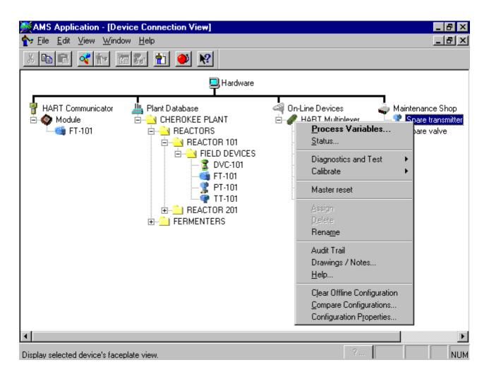
Figure 1. AMS gives users the ability to communicate with live instruments in the field, and to access all instruments' historical records. By simply clicking on an instrument icon all information, including device status, is instantly available.
